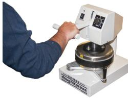
6. Once the set time has elapsed, the timer will sound. Press down on the handle once more to release the crust from the upper platen then raise the handle to open the press.
