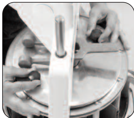
Figure 1: Remove pan, completely loosen both Black Knobs. Do not Drop the Divider Head as damage may occur!
